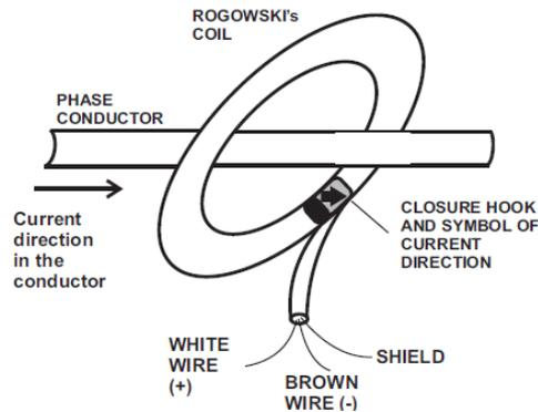
Rogowski's coil (accessory RC-V400-100) have been designed for accurate nonintrusive measurement of AC, pulsed DC or complex waveforms.
