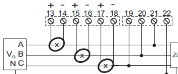
**3.1. 3-phase without neutral insertion (4-wires insertion)**
