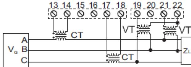
**2.8. 4 wire with neutral insertion with CTs (4 wires insertion)**
